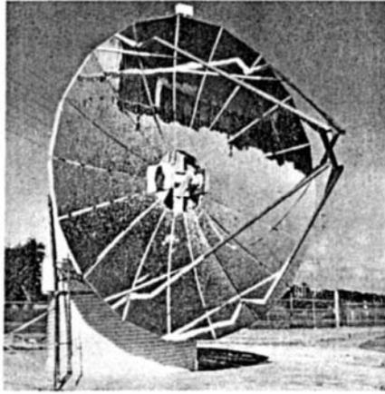
**Fig. 49.12** Commercial paraboloidal solar concentrator. The receiver assembly has been removed from the focal zone for this photograph. (Courtesy of Omnium-G Corp., Anaheim, CA.)
